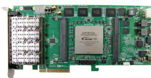
Receiving board aggregate synchronised data to feed GPU filter farm
