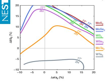
Intersection contours of the 2H and 1T' energy surfaces when varying the rectangular lattice constants a and b [3].
