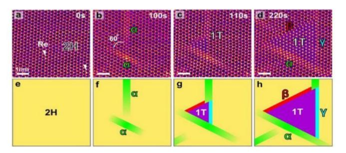
An alternative approach to induce a SPT by Rhenium (Re) intercalation and thermal annealing in  $MoS_2[5]$ . National Enterprise for nanoScience and nanoTechnology
