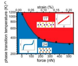
Modulating the phase transition temperature of  $MoTe_2$  by strain [4].
