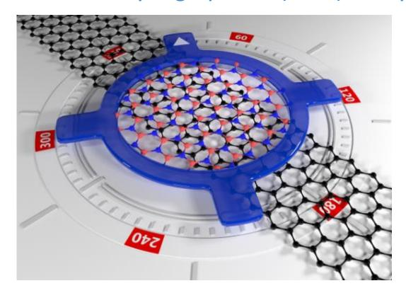
**Twist angle** → new degree of freedom induces several angle dependent properties in tBLG → vastly different electronic behavior that depends sensitively on the angle between the layers
