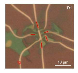
30°-twisted bilayer graphene from chemical vapor deposition (CVD):
