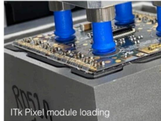
ITk Pixel module loading
